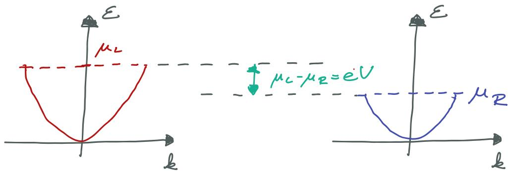
APPLYING POSITIVE VOLTAGE ON A METAL :
