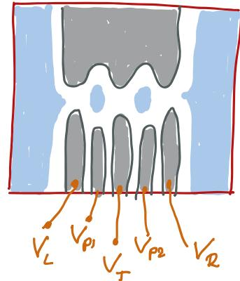
$$E_{\text{TOT}} \approx \frac{Q_1^2}{2C_1} + \frac{Q_2^2}{2C_2} + \boxed{\frac{1}{2} \frac{Q_1 Q_2}{C_m}} - Q_1 V_{G1} - Q_2 V_{G2}$$
